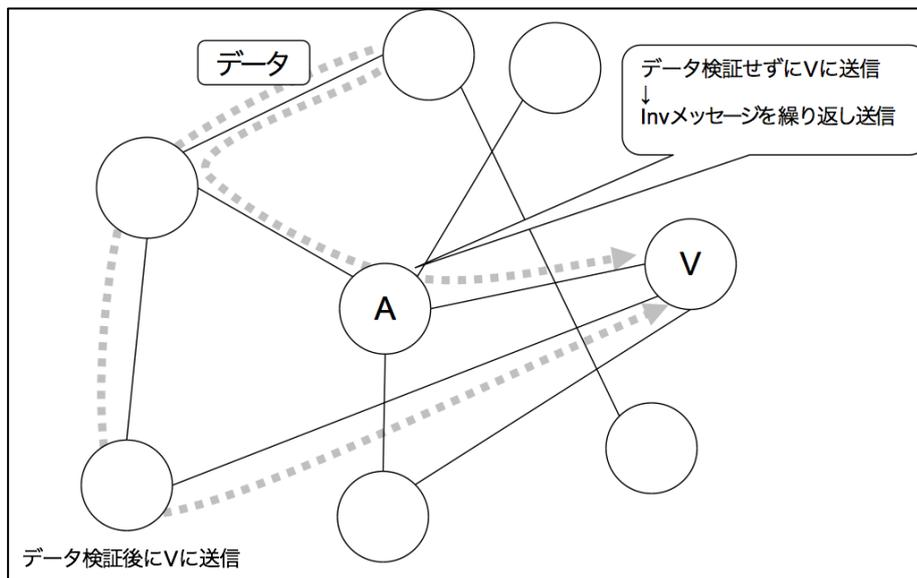
Figure 6-11: Schematic overview of tampering attack
