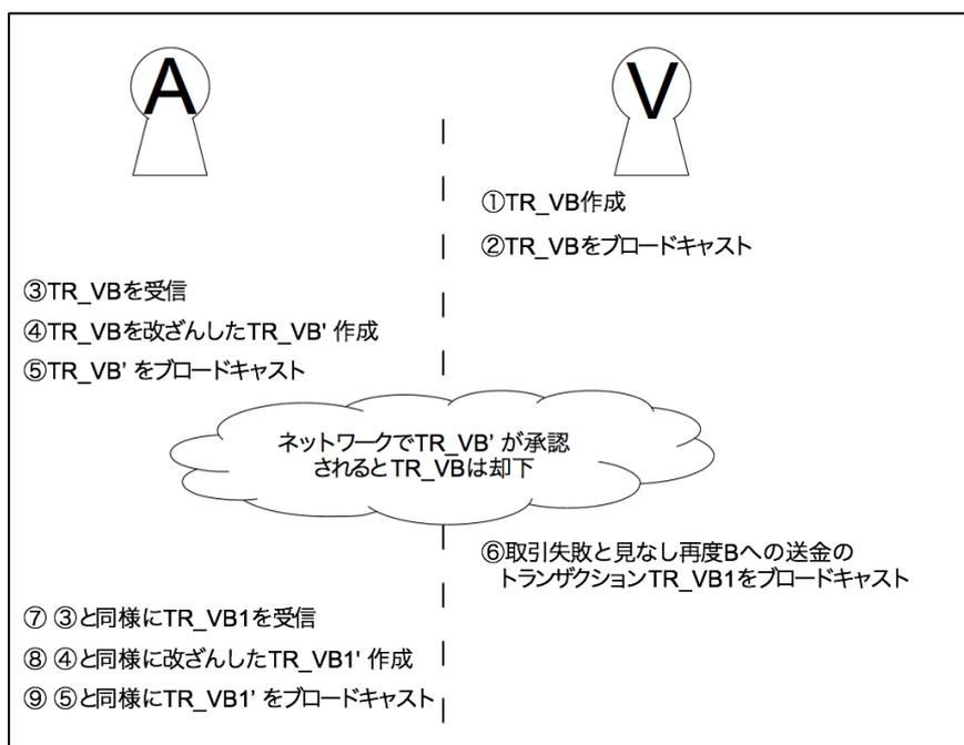
Figure 6-8: Schematic overview of transaction malleability
